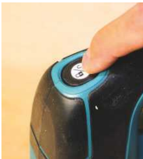
▲ You need to press this button to unlock the saw before it can be used
